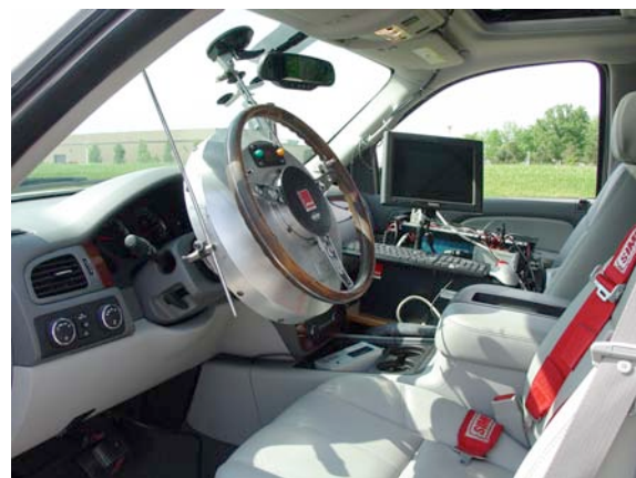
Data acquisition system and robotic steering wheel controller.
