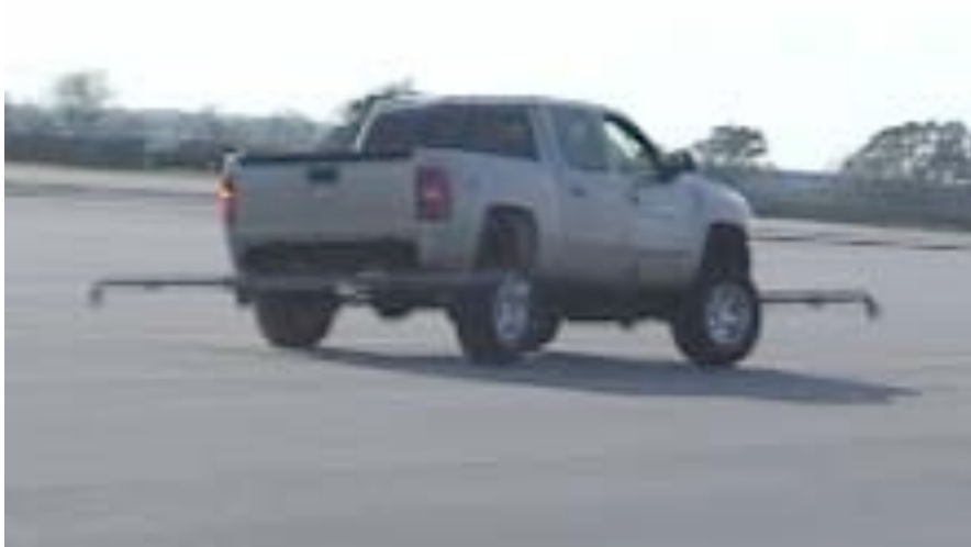
The Pro Comp equipped 2008 Silverado during Electronic Stability Control System testing.
